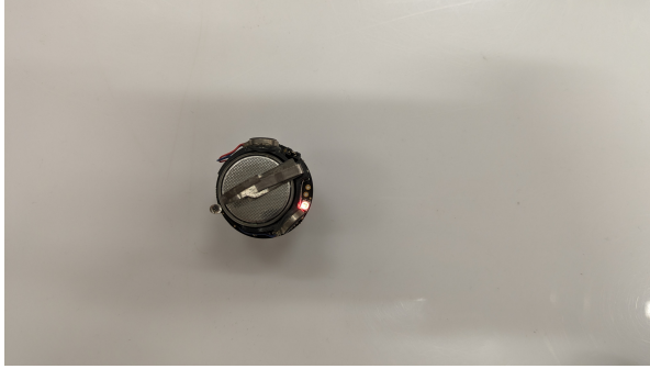
(a) Single Kilobot detecting no neighbours indicated by red LED light.
