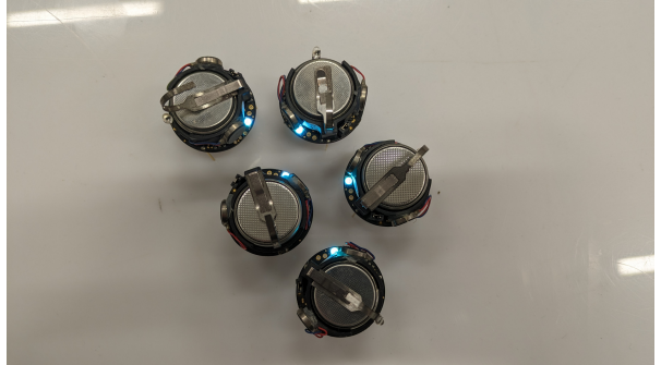
(d) Five Kilobots detecting three or more neighbours indicated by white LED lights.
