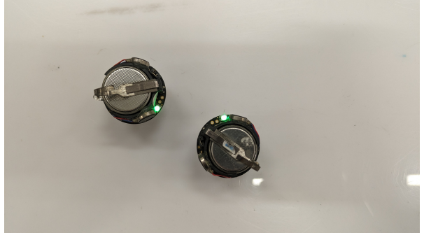
(b) Two Kilobots detecting a single neighbour indicated by green LED lights.
