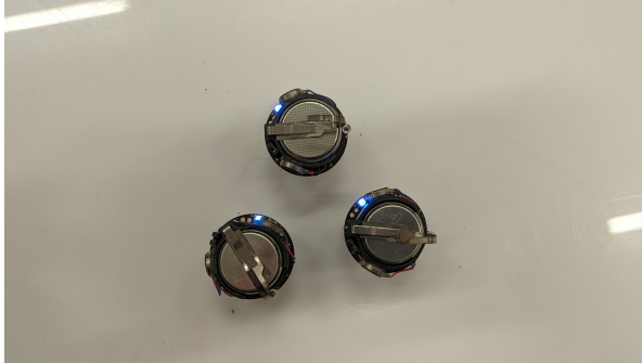
(c) Three Kilobots detecting two neighbours indicated by blue LED lights.
